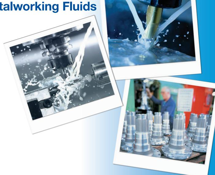
Tech Cool metalworking fluids are a stable, emulsion blend of mineral oil, corrosion inhibitors, and extreme pressure additives. When mixed with water, they form a translucent solution that provides cooling, lubricity, and protection. Tech Cool metalworking fluids offer a cleaner metalworking operation even in high speed/high pressure machines.
