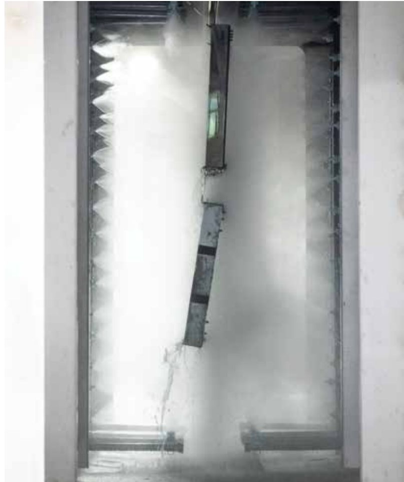
Newly installed 5 stage washer and paint line.
