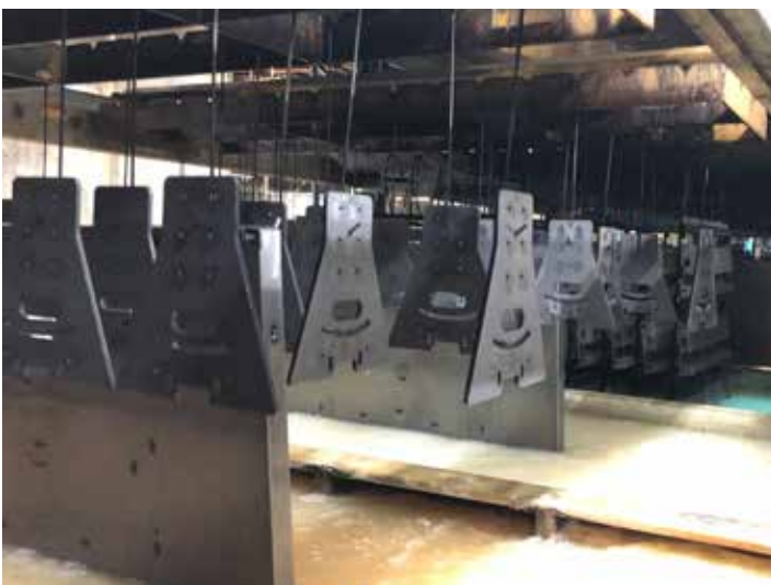
Gardobond 24T zinc phosphate pretreatment prior to cathodic epoxy ecoat paint.
