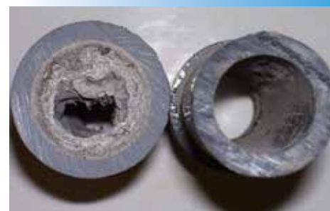
Cross-section of a pipe before (left) and after (right) descaling
