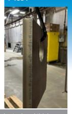
Scale removal on 1/2 inch steel and thicker
