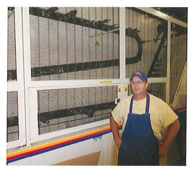
Machinist Bruce Reisenauer uses Chemetall Tech Cool 35052 semisynthetic at 8-percent concentration to machine trunnions, axle pads, and roller, upper-link, trans, cab, and engine mounts on a Mazak MazaTech FH-880.
