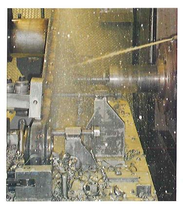
Before 2012, CNH Fargo used high-lubricity synthetic coolant that left sticky residues that fouled the automated tool changers and caused corrosion. Chemetall's Tech Cool 35052 (pictured above) is a high-lubricity, semi-synthetic coolant that demonstrated no corrosion or sticky buildup during testing.
