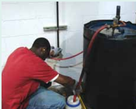
Fisher-Barton uses a dispensing station to provide consistent mixtures of oil and water for each operation throughout the plant.
