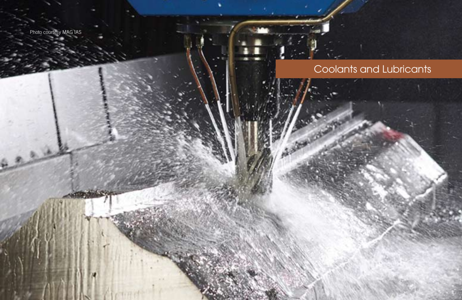
Titanium aerospace component machined using MAG Cyclo Cool metalcutting fluids specifically designed for high-heat alloys.
